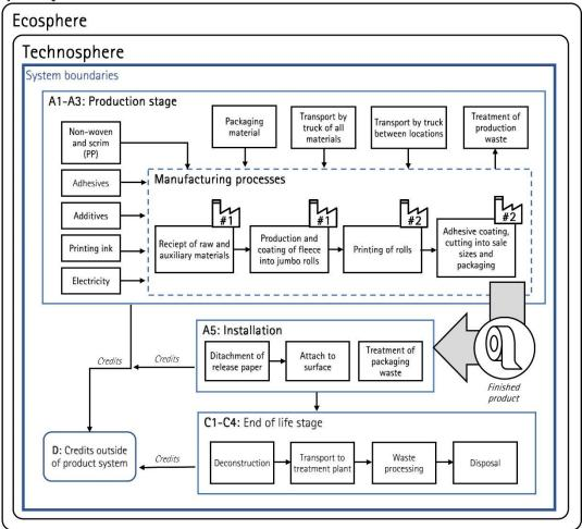
Each processing step within the system boundaries is marked with an icon and number (#1, #2, etc.), indicating the specific production site where it occurs. The system boundaries cover the following modules:
